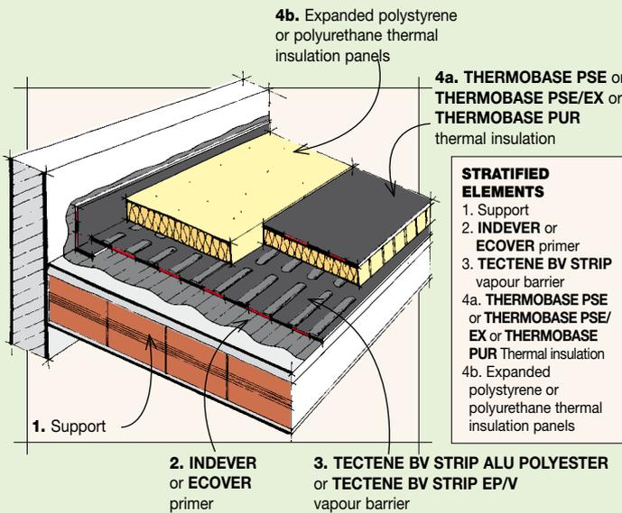
**VAPOUR BARRIER WITH INCORPORATED HOT-MELT ADHESIVE FOR THE ADHESION OF THE LAYER OF THERMAL INSULATION AND HEAT-BONDING OF HEAT-RESISTANT INSULATING PANELS OR THERMOBASE PUR PANELS**
