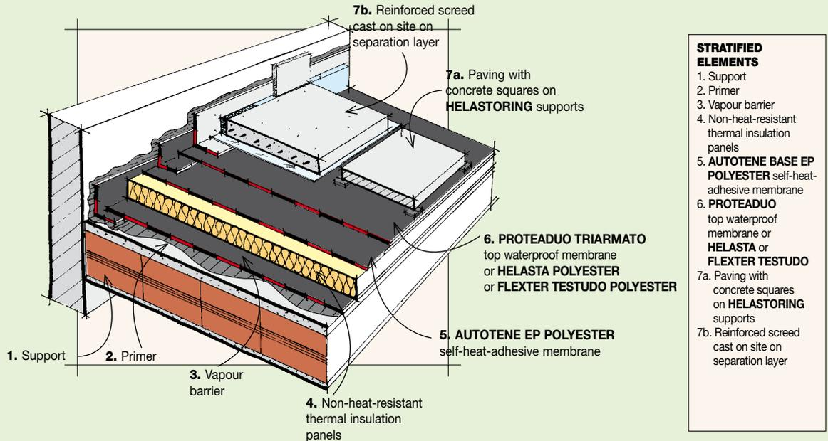
For heat-bonding the membranes onto heat-sensitive insulating materials (expanded polystyrene either extruded or sintered) they must first be protected. For laying the membranes with adhesion onto the expanded polystyrene, either extruded or sintered, a special self-heat-adhesive substrate of AUTOTENE BASE EP POLYESTER must be used, which is applied dry onto the insulation and subsequently adheres on its own due to the heat produced by the heat-bonding of the upper layer that is stuck on top.
