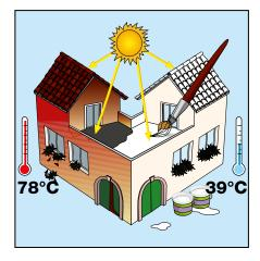
Waterproofing and protecting complexshaped concrete structures where the use of rolls of prefabricated polymer-bitumen membrane is difficult and where the presence of heat and naked flames increases the risk of fire.
