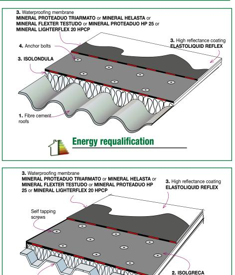
For thermally insulating trapezoidal or corrugated panel roofs, use ISOLGRECA or ISOLONDULA, themselves protected by a slated waterproofing layer to which **ELASTOLIQUID REFLEX ultrareflective coating** can be applied.
