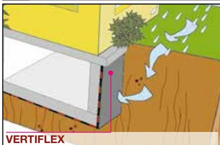
**VERTIFLEX POLYESTER** is the membrane designed by Index to solve waterproofing application problems of foundation walls. In these cases, the membranes to be used mainly for lining roofs, can present greater difficulties which prevent correct execution and adhesion during torching.
