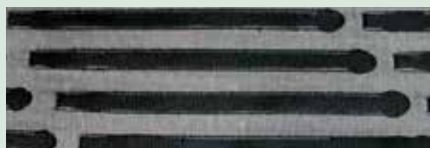
ADHESIVE STRIPS ON SAND BLASTING.
