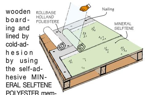
The same technique can be used for refurbishments and in all situations where an exposed flame cannot be used. **ROLLBASE** can be dry laid as a sliding layer on flat roofs ballasted with gravel and terraces which can be walked on. It can be spot-bonded with molten bitumen or with cold adhesives and the bond is much stronger and lasts longer than that obtained between oxidised bitumen and membranes containing polymer-bitumen.
