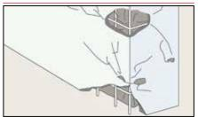
Some concrete repair work requires the application of large thicknesses without using formwork. Repairs to corners of beams or pillars, front cornices, and the formation of wall-floor joining mouldings require highly thixotropic mortar, with compensated shrinkage in order to avoid cracks and shrinkage hairlines.
