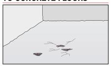
In more serious cases of concrete repairs, when greater thicknesses are required, you need to use mortar that can be poured into formwork, with high strength and fluidity. It is easier to repair deteriorated concrete floors using pourable mortars.
