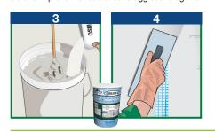
In the renovation of old paving, apply the adhesive FLEXBOND or GRANICOL AB RAPID after the hardening of the waterproof layer.
