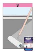
always be applied on the film of the perfectly dry first coat. Never exceed a dry film thickness of 0.3 mm for each coat (about 0.500 kg/m² per coat) so as not to hinder the evaporation of the water contained in the liquid bitumen product, which
