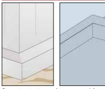
Concrete structures of terraces and foundations without joints or built on surfaces made up of filling materials are subject to constant settling, which causes cracks along the lines with the highest tension. It is therefore necessary to use elastomeric bitumen waterproofing products to protect them from infiltration problems when polymer bitumen membranes cannot be used.
