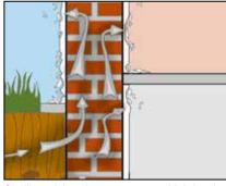
Capillary rising damp transports high levels of salts such as sulphates, chlorides, nitrates, etc. with it, which crystallise producing surfacing salts. The tension caused by the crystallisation
