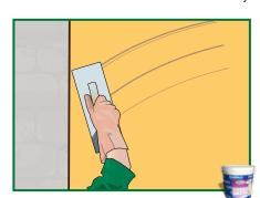
Avoid working on walls exposed to sunlight during the hottest periods of the day. Old paint and plastic coatings must be clean, free of clefts or cracks and adhere properly to the surface.
