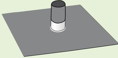
VERTICONNECT is a vertical connection with sleeves, which can be adapted for running cables in waterproofing elements with polymer-bitumen membranes.
