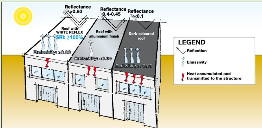
Temperature levels reached by the waterproof covering with different surface finishes exposed in the same conditions to summer solar radiation
