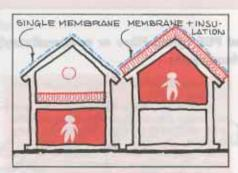
that where warm surfaces are subjected to cold air or cold surfaces are subjected to warm air, condensation can form. Therefore great care must be taken to ensure correct thicknesses of insulation and the presence of adequate ventilation where necessary.
