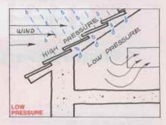
All these phenomena are connected with wind. Laboratory experiments carried out on clay tile roof have verified that, contrary to what is believed, wind speed in itself has very little influence. In fact it is the creation of different internal-external pressure which contributes most significantly to water penetration. In fact with a wind speed of 30-60 Km/H it is possible to create serious infiltration over the whole roof.
