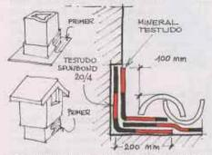
The alternative method is for a purpose made recess to be provided at the foot of the chimney which would be waterproofed as shown in the
