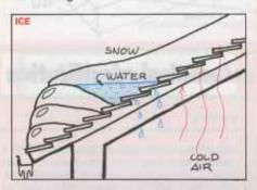
The ice which builds up could lift tiles allowing considerable water infiltration.
