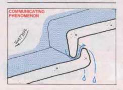
up on the roof can result in the passage of water between the two elements of the tiles.
