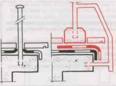
6 Breakage of waterproof covering caused by movement due to a lack of expansion joint. Repair: creation of a correctly constructed expansion joint using HELASTA P and MINERAL HELASTA P.
