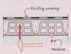
Double roof with non-ventilated interspace can be the seat of condensation which is at times mistaken for leaks in the waterproof covering; in this case as well, it is a good idea to bore air holes.
