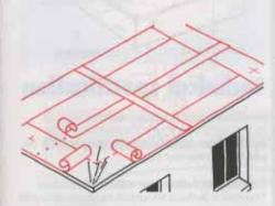
4 Waterproofing beneath a paved area of flat roof which is below threshould level.
