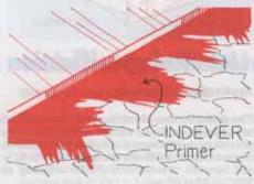
When a few breaks are present on the covering due to concrete shrinkage or to broken slope blocks, it is possible to repair the old covering in the following way before applying the new membrane.
