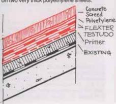
In re-making tiled roofs it is better to insert waterproofing and insulation before setting the new tile layer. The surface should be carefully cleaned and made level.
