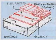
Gravel Stratum: a layer of non-woven polyester, 200 gr/m² type filtro with unbonded 100 mm overlaps will be loose laid on he membrane, then a washed gravel layer (granulometry 16/32 mm) 40 to 50 mm thick should be spread over the whole surface.
