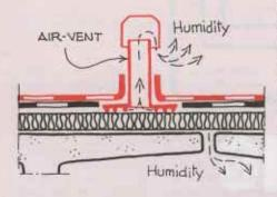
In case of insulation without a vapour barrier placed under paving on residential roofing, where the deck is on site cast concrete with hollow pot construction it is often better to strip off the complete covering in order to avoid the risk of trapping large quantities of moisture, between the insulation and the surface of the deck.
