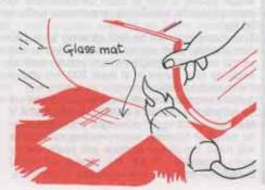
When there are blisters (usually multilayer coverings composed of bituminized felt paper), these should be cross cut and flattened, the area then painted with a coat of bituminous primer and a strip of FLEXTER TESTUDO fully welded which overlaps 100 mm beyond the surface cut.
