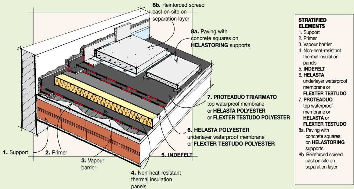
For heat-bonding the membranes onto heat-sensitive insulating materials (expanded polystyrene either extruded or sintered) they must first be protected.
