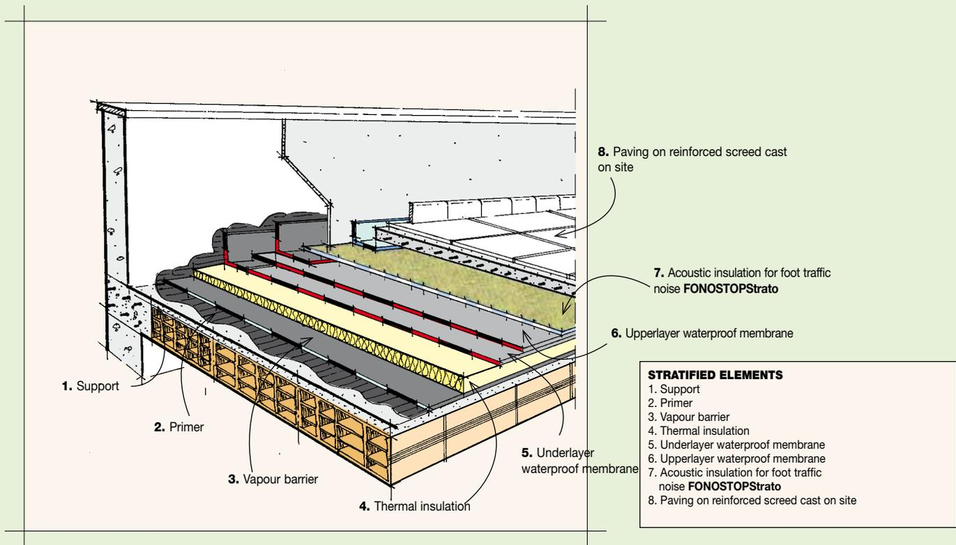
The load-bearing structure of terraces usually consists of floor slabs that are heavy enough to ensure observance of the legal limits specified for acoustic insulation against airborne noises.
