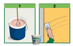
Rendered surfaces should be trowelled and regular for easier application. In summer, surfaces should be wetted. Avoid working on walls exposed to sunlight during the hottest part of the day. If necessary, provide a coat of primer to make the base uniform.
