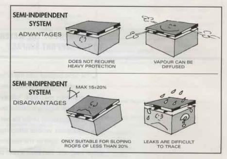
Leaks in the covering are difficult to trace. The semi-independent system is generally used on open coverings on unstable or damp laying surfaces. The mechanical fixing method merits separate consideration which is unbeatable for its practicality and effectiveness on certain surfaces.
