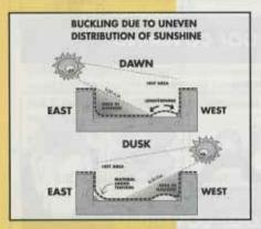
displacement of the covering and/or adjacent layers in a rippling movement are called buckling.
